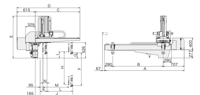
■ Operator Side Discharge Direction [mm]
